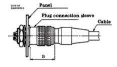
Hold the plug connection sleeve B and pull the sleeve straight.
