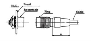
Hold the plug at point A, align the plug guide with the receptacle guide, and push the plug straight.
