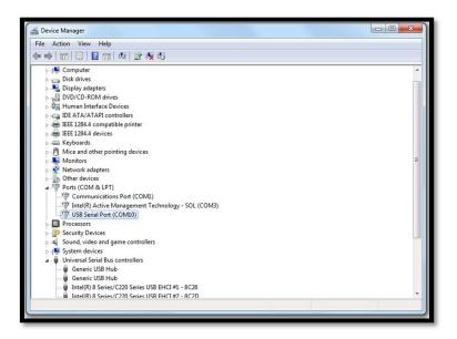
4. Under "Ports" the USB Optical Probe should be listed as "USB Serial Port (COM X)" where the (X) means the Port Number automatically assigned by the PC and it can be any number. This COM port number will be selected in the Meter Reading Software to start communication between the electric meter and the USB optical probe.
